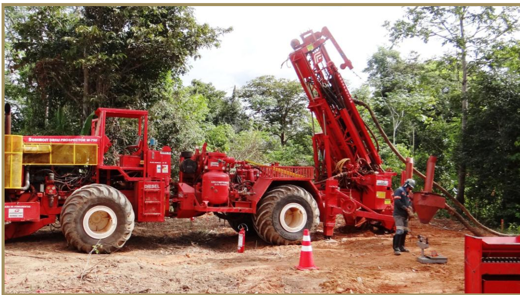
Figure 10: Reverse Circulation (RC) Drill Rig utilised in Ana Prospects Drilling – Prospector W-750 drill equipped with PCM 900 x 350 psi compressor and booster compressor.
