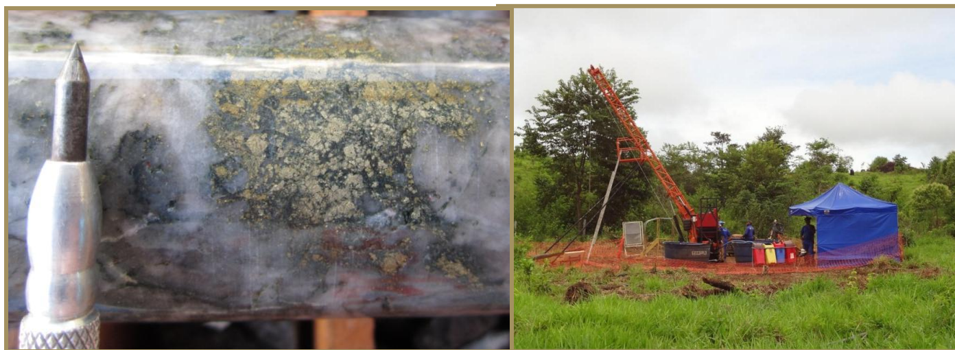
Figure 12: Ana South – Hole ANS025. Zone of intense silicification with disseminated pyrite and chalcopyrite with localised strong propylitic alteration.
