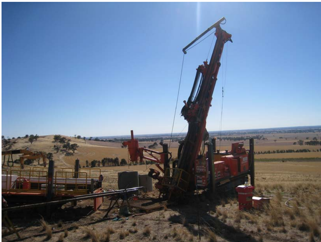
Figure 3 – Drilling geotechnical hole GTC2 at Golden Camel
