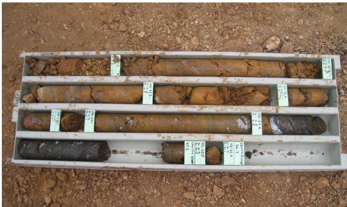
Fig.2 - Transition of brecciated chert mineralisation from oxide to fresh sulphides within EXP01 including 1.4m cavity (65.3m - 66.7m) which was a common occurrence within the mineralised zones (EOH 72.4m).
