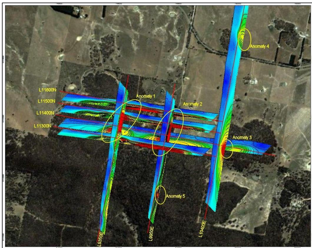
**Figure 1:** Chargeability anomalies identified along several east-west and north-south IP survey lines
