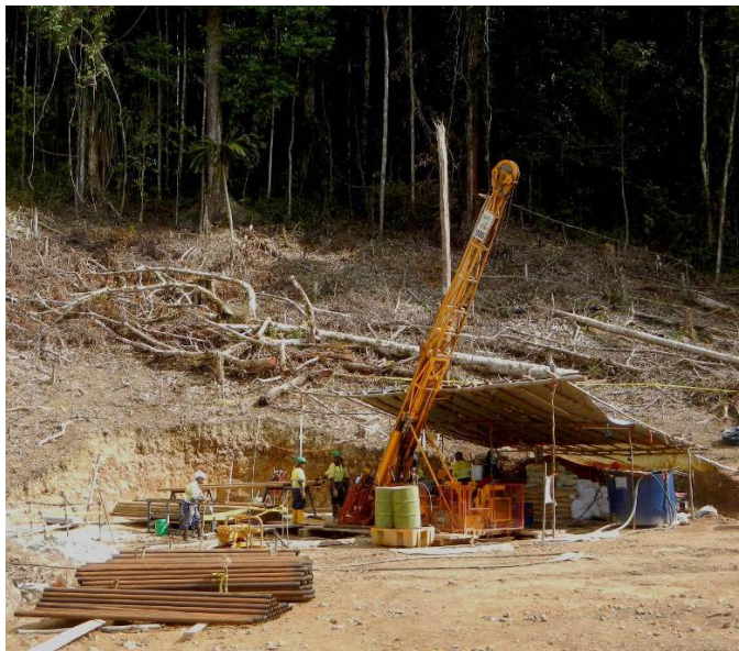
Photo 1: Diamond drilling at KIKDH001 drill pad
