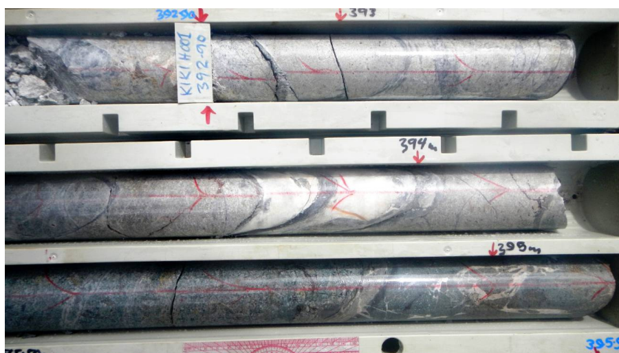
Photo 3: Phyllic altered quartz diorite with anhydrite and quartz sheeted veins, 1-2% disseminated sulphide through groundmass and along vein margins + irregular sulphide blebs (<5mm).
