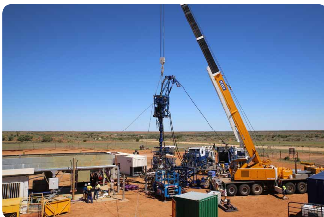
Right: The coil tubing unit in operation removing the plug from Habanero-1
