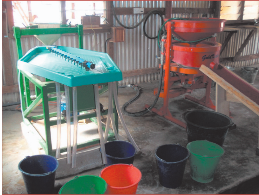
Figure 15. Exploration gravity concentrator for bulk alluvial samples
