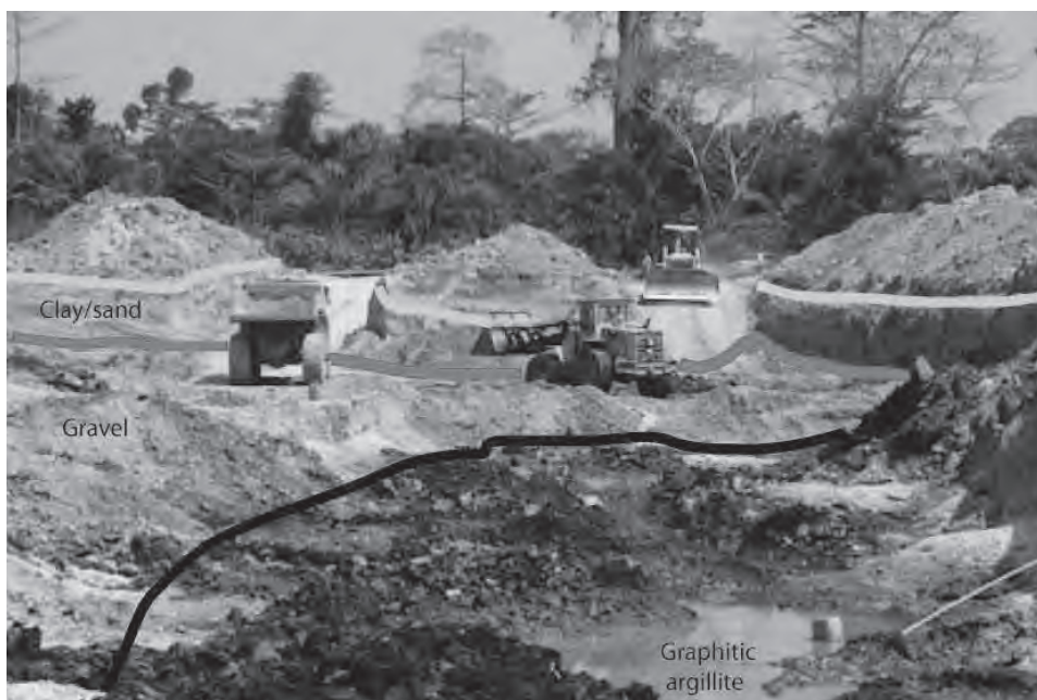
Figure 4 THE Kashmir trial pit. Lines show the lithology boundaries. Graphitic argillites overlain by 02-5m of auriferous .gravels and 2-5m of clays and barren sands
