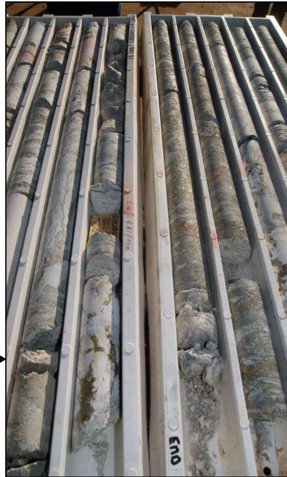
12HOD012 drill core showing heavy matrix sulphide
