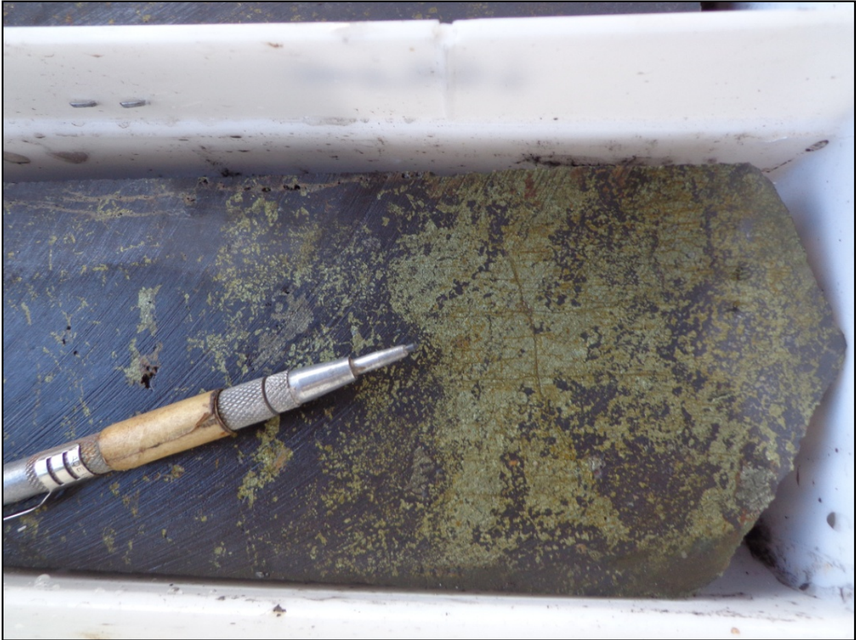
Photograph 2 - Chalcopyrite and magnetite skarn mineralisation.
