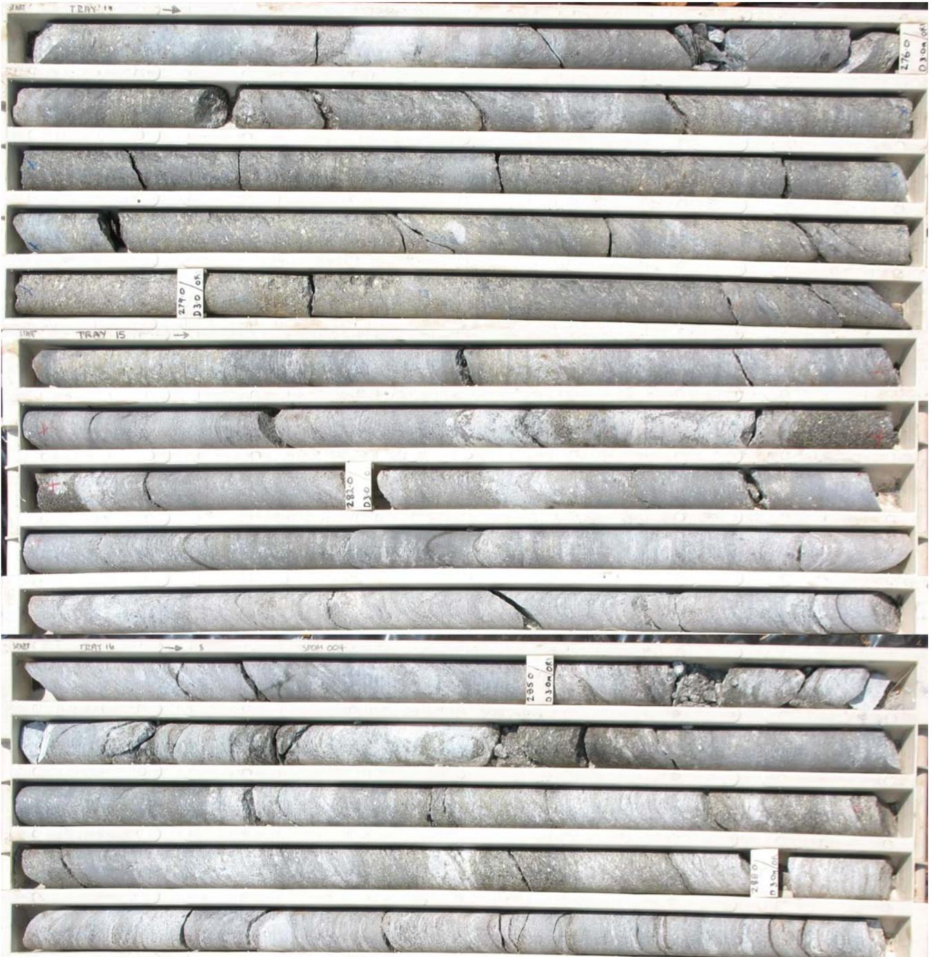
Photograph 1. One Mile Mining Lease – Photograph of core from hole SPOM004 for the interval 275m to 289m (Trays 14, 15 and 16). The interval of semi-massive sulphides in the top two trays between 275.6m and 283m of 7.4m averages 0.42% Cu, 0.50g/t Au and 1.64% Zn.
