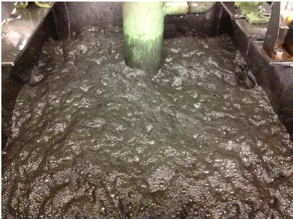
Figure 2. First rougher concentrate, assaying 5380g/t Ag with 68% Ag recovery
