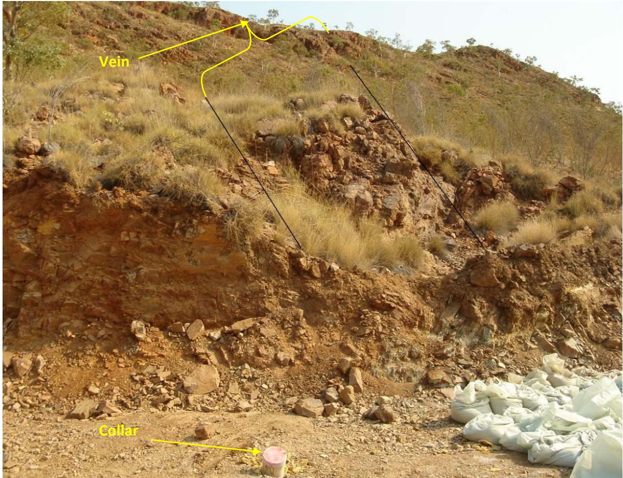
Figure 3 – Collar of Hole JT11RC01 relative to outcropped cross vein being responsible for the intercepted shallow copper mineralization (looking northwest).
