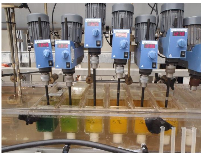
Plate 1: TNG/METS TIVAN – Stripping mixer/settler cells under controlled temperature conditions
