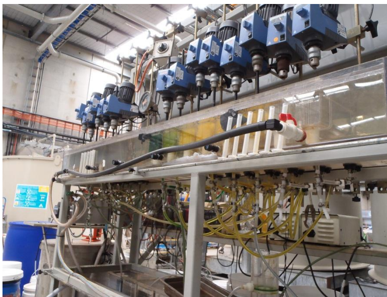
Plate 2: TNG/METS TIVAN – Extraction & Stripping sections including organic recycle & individual cell flow control
