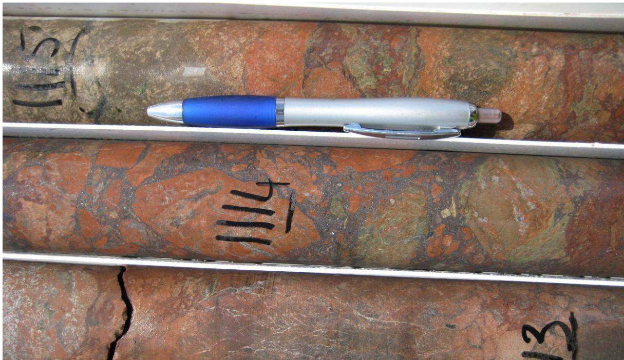
Figure 7: Detailed photo of brecciated host volcanic (red) with mineralized (pyrite-chalcocopyrite) hematite matrix (dark grey). (NQ drill core)
