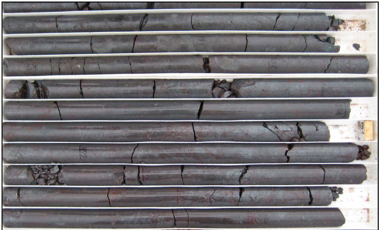
Figure 2: Hematite breccias, typical of the 242m zone intersected in VUD 9 (NQ 2 drill core).
