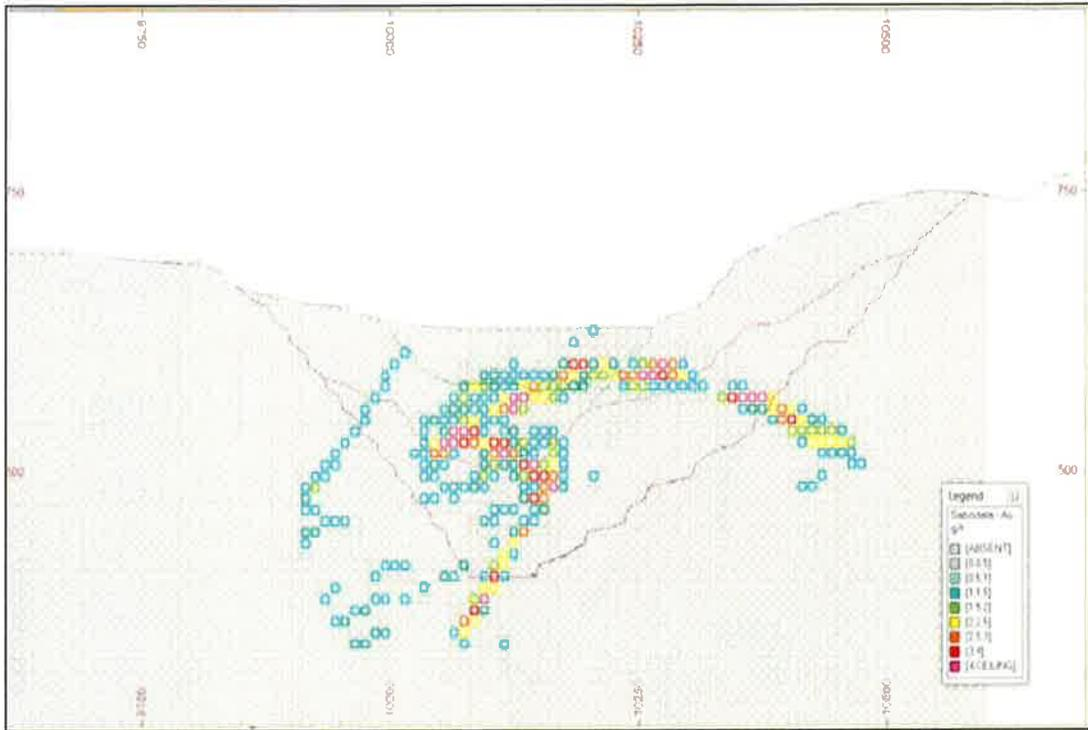
Figure 15.3 Sabodala, Sutuba Ultimate Pit Design - Long Section at 10100E, looking East
