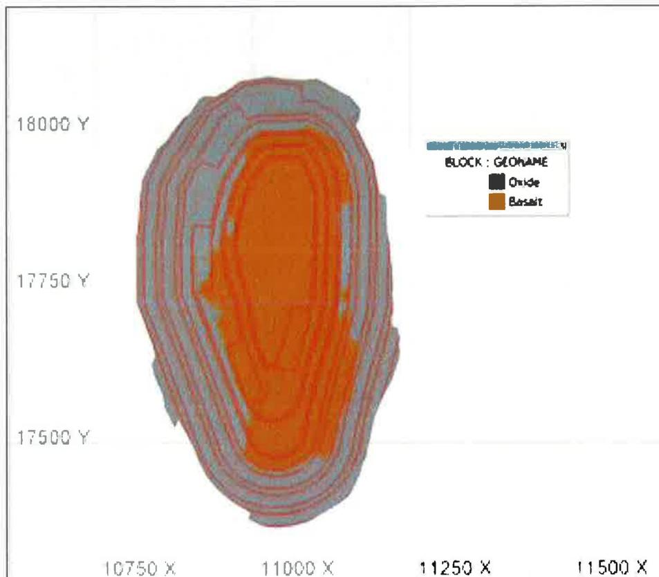
The Niakafiri pit will be mined in a single phase (Figure 15.6 and Figure 15.7). The ultimate pit contains 30.4 Mt of rock including 22.6 Mt of waste and 7.8 Mt at 1.14 g/t Au of Proven and Probable Mineral Reserves resulting in an average 2.9:1 waste to ore strip ratio. The design was developed using a cut-off grade of 0.5 g/t Au for fresh rock and 0.35 g/t Au oxide (refer to Table 15.1).
