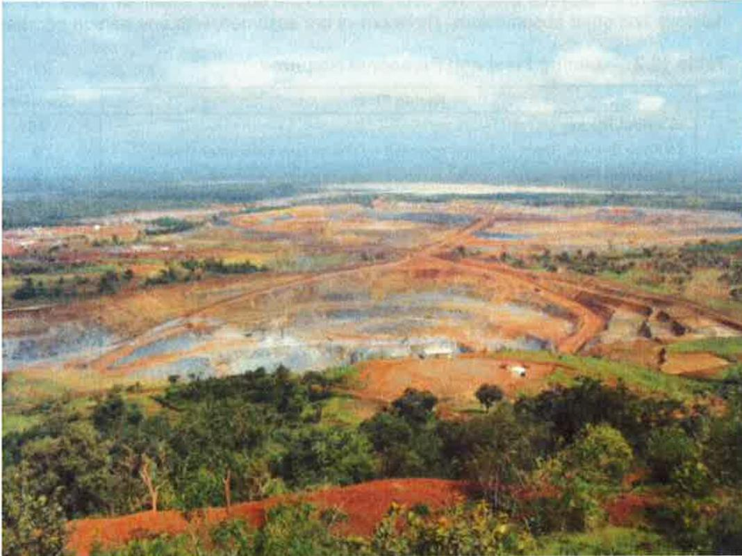
The mining method utilized is conventional truck and shovel open pit mining. The mining operation is effective at selectively separating ore from waste, and in separating the four ore categories that are stockpiled if not immediately milled. These are namely; high grade, medium grade, low grade and marginal as defined in Table 16.1.
