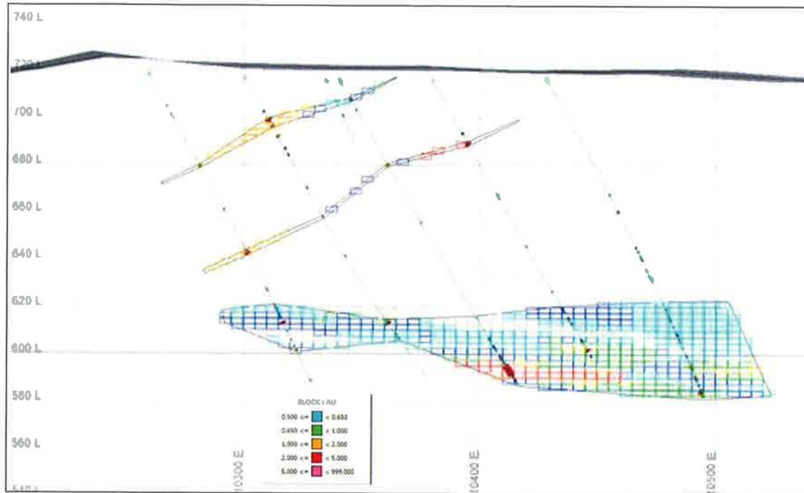
Figure 14.3 Cross Section through Soukhoto Deposit, (18420N)
