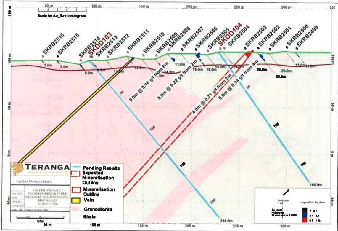
Figure 9.6 Section showing Mineralization Encountered in SKRC255 and KRC257
