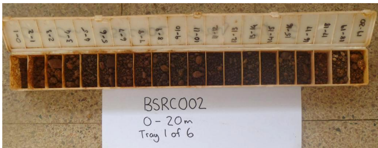
Figure 4. BSRC002, goethite / hematite rich iron formation interval of 14m @ 41.96% Fe from 2 to 16m
