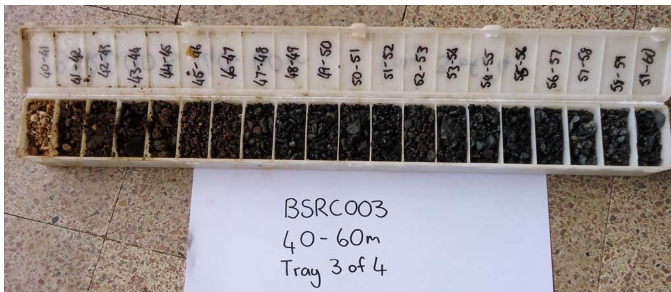
Figure 5. BSRC003, magnetite bearing iron formation (part of intercept 30m at 25% Fe)
