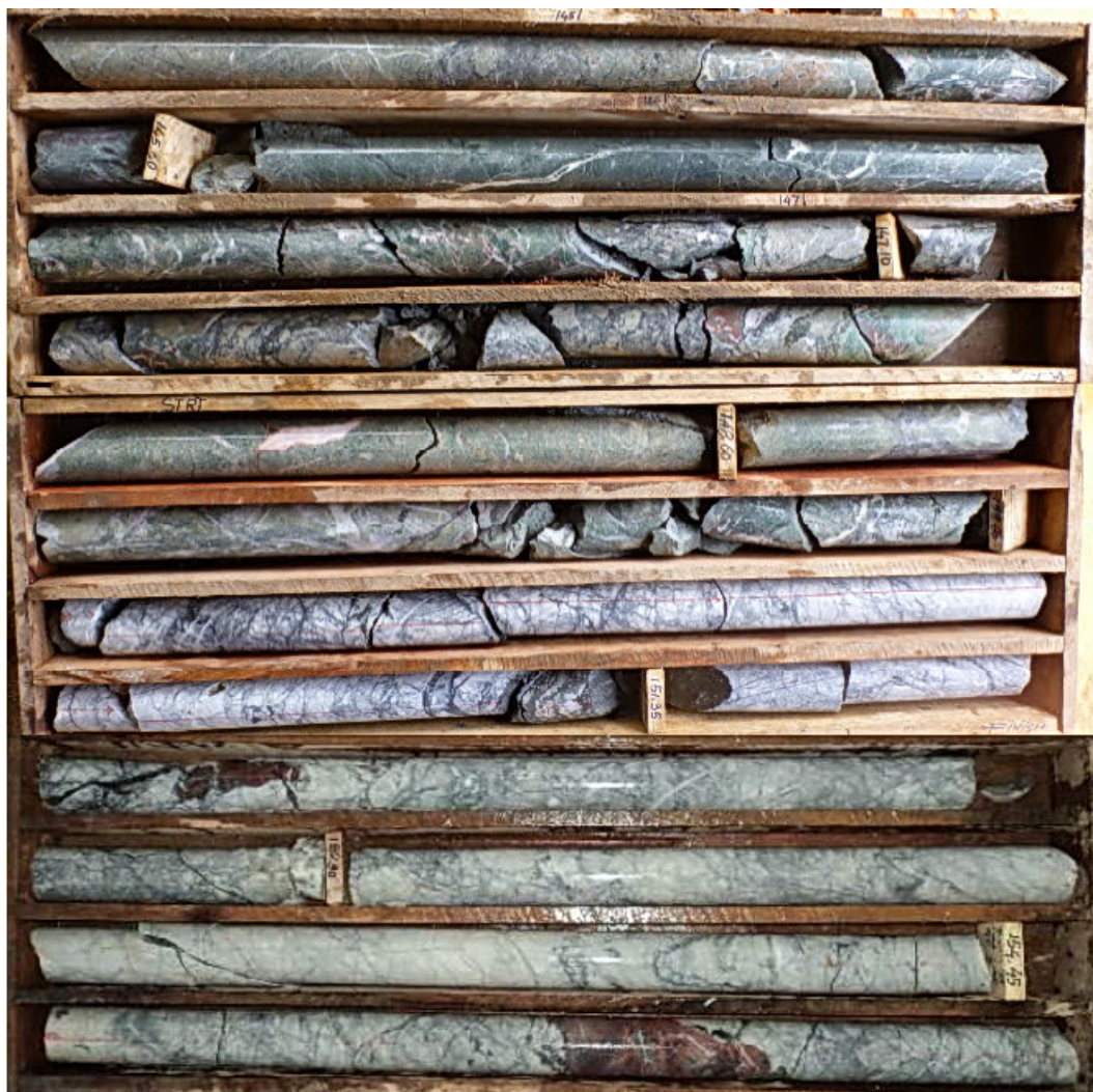
Figure 10: Core interval 144.3 - 155.5 m showing intersection from endoskarn in microdiorite through limestone (marble) and porphyritic diorite mid-section of drill hole. Note fracture pattern through rocks and high core recoveries achieved in drilling in these rocks.
