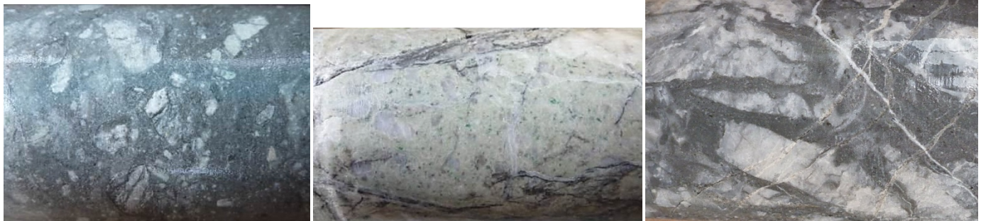
Figure 4: (L) Intrusive breccia, 128 m; (C) Sheared granodiorite with sulphide, 130.23m; (R) Brecciated quartz vein with silica-pyrite fill, 130.6m
