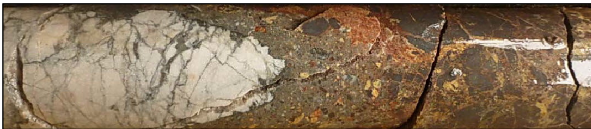
Figure 11: Intersection between microdiorite breccia and limestone at footwall contact in Hole PNGD021 at 53.m depth.
