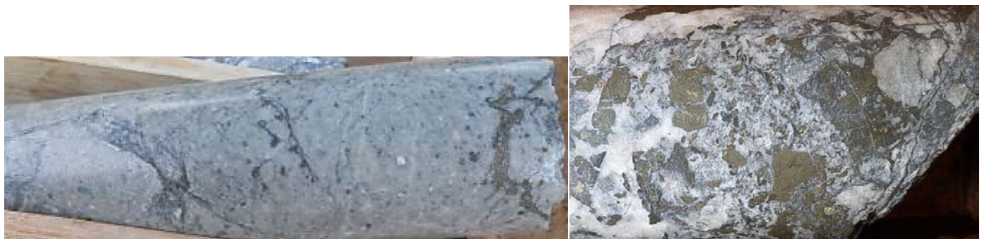
Figure 5: (L) Altered microdiorite, 133.6 m; (R) Limestone (marble) - pyrite breccia, 157.3m
