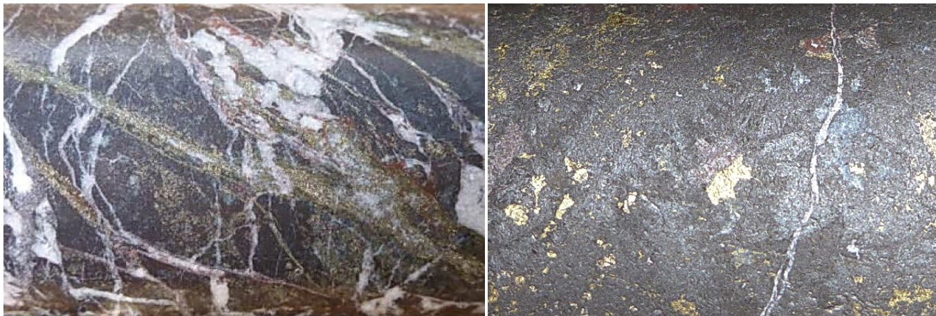
Figure 7: (L) Altered microdiorite with late sulphide fill in veins, 166.5 m; (R) Massive magnetite rich endoskarn with chalcopyrite and pyrite in matrix, 176.5 m.
