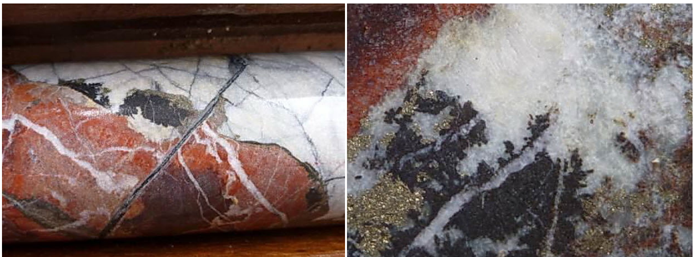
Figure 6: (L) Altered microdiorite in contact with limestone; (R) Detail of photo left showing magnetite-pyrite-hematite alteration, 159.95m
