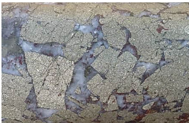
Figure 8: Coarse pyrite at limestone (marble) contact with microdiorite, 192.4m.
