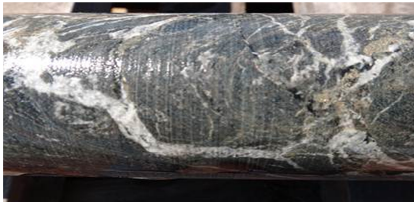
Figure 1 – Quartz/carbonate stringers in foliated and chloritic mafic rock at 390.8m
