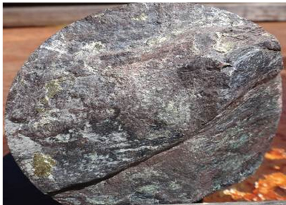
Figure 3 –Hematite/magnetite/chlorite banding in metasediment, minor chalcopyrite at 415.4m
