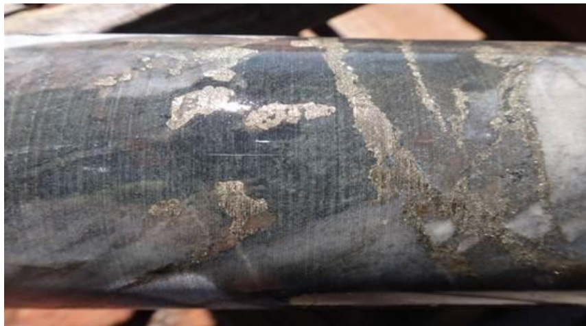
Figure 3 –Pyrite and chalcopyrite in stringers and on joint planes in black shale rock at 415.4m
