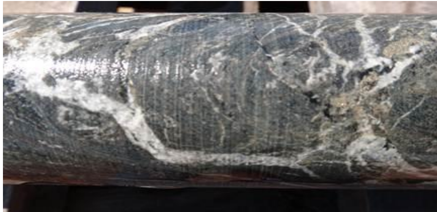
Figure 2– Quartz/carbonate stringers in foliated and chloritic mafic rock at 390.8m
