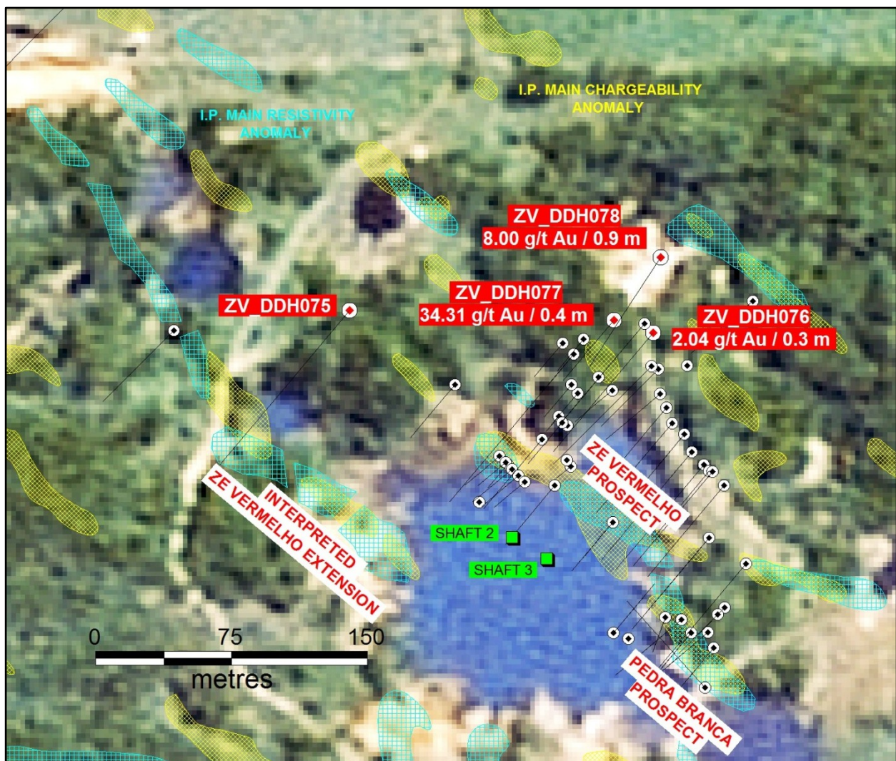
Figure 2: Plan map of the Ze Vermelho drill holes and main I.P. anomalies (resistivity and chargeability).
