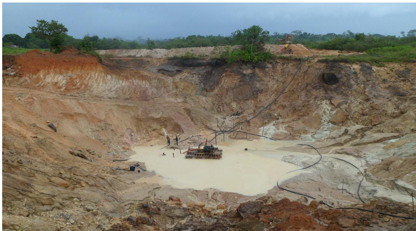
Figure 6: Tambaqui west pit undergoing dewatering.
