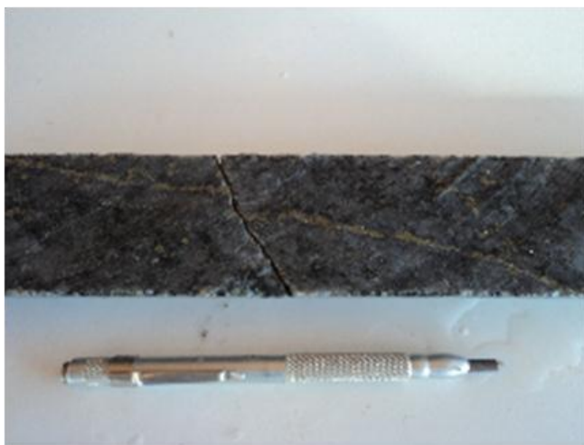
Fracture filled by pyrite with 3mm wide, position 93,22 meters and N52E/43SE
