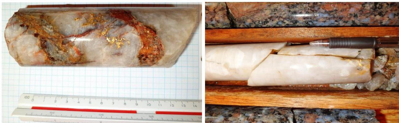
**Figure 6: Free gold from diamond holes ZVDDH024 (from 37m) and ZVDDH025 (from 47m)**
