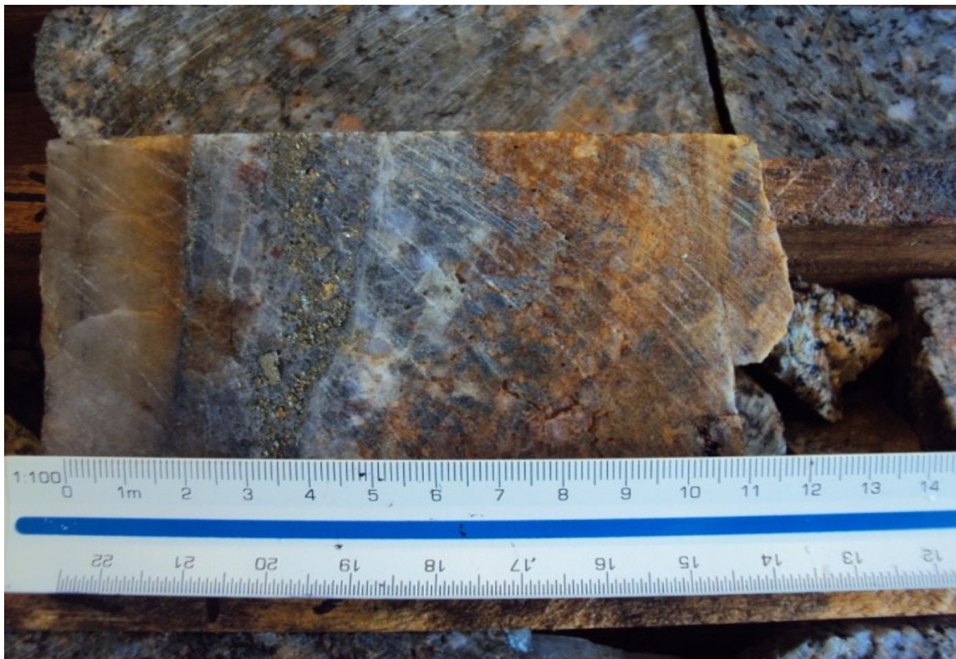
Figure 3. Hole ZV-DDH031: 1cm of nearly massive pyrite band in quartz vein; from 40.20 metres.
