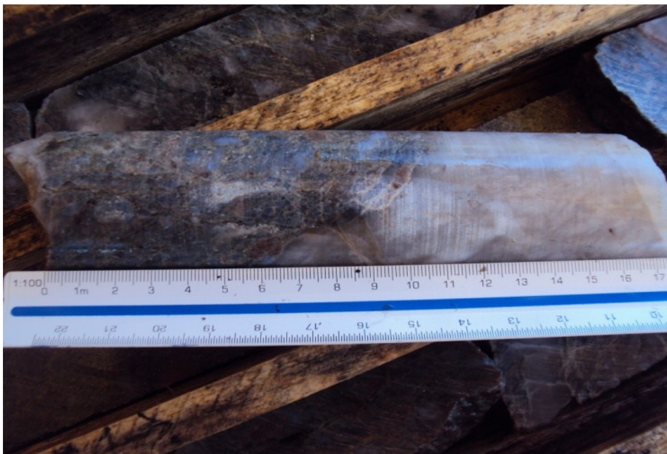
Figure 1. Drill Hole ZV-DDH029: Mylonite (grey) in contact with quartz vein (white) showing pyrite dissemination along the mylonitic foliation; from 42.85 metres.
