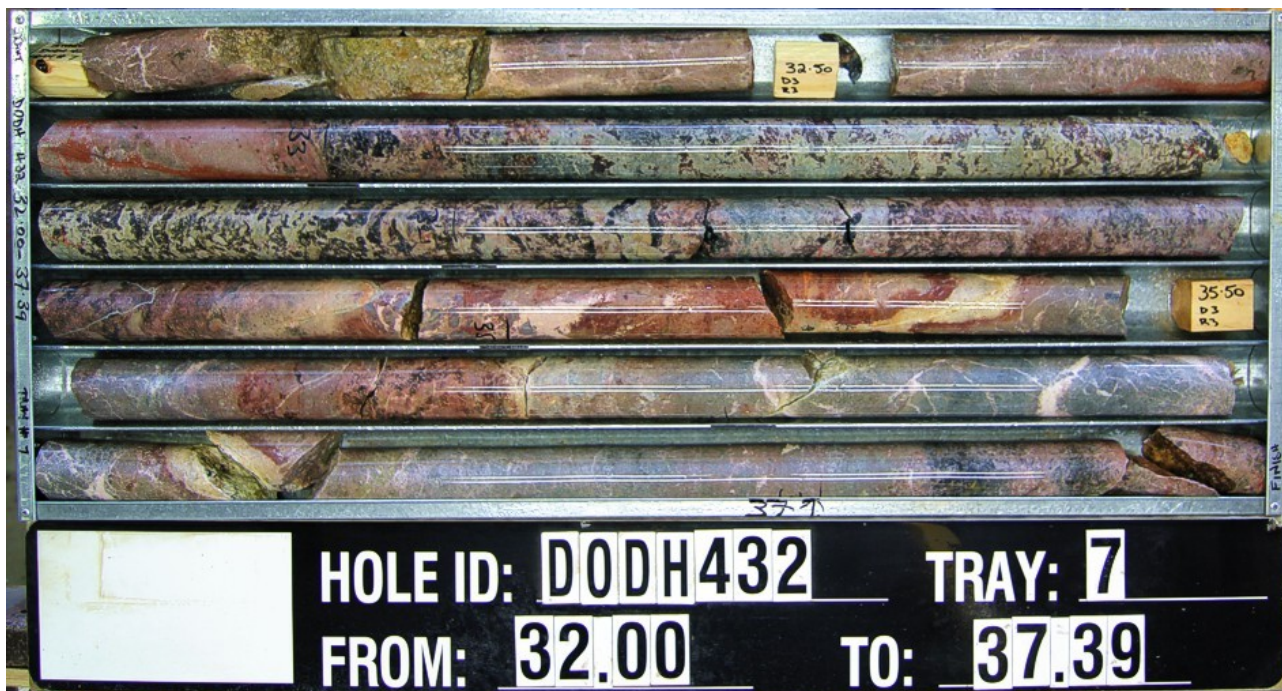
Figure 1: Diamond drill core from DODH432, showing the highly-altered zone hosting high-grade gold, silver, uranium and tellurium mineralisation at 36m
