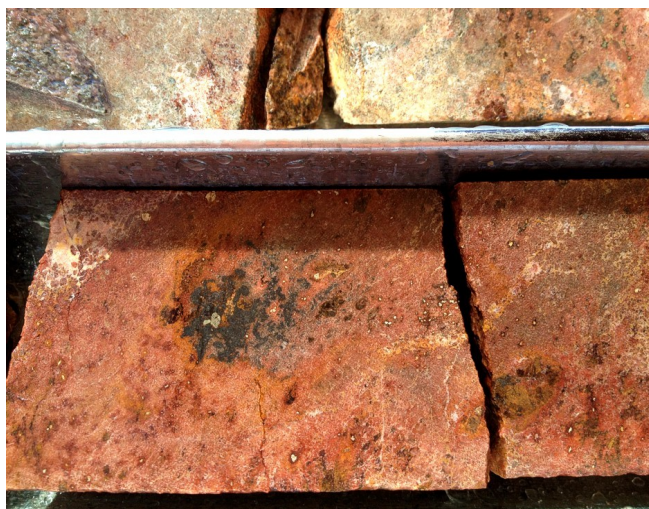
Figure 2: Diamond drill from DODH432, showing close-up of uranium mineral (carnotite) at approximately 36.4m.
