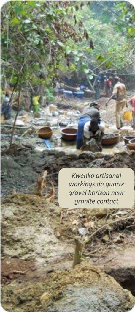
Kwenko artisanal workings on quartz gravel horizon near granite contact
