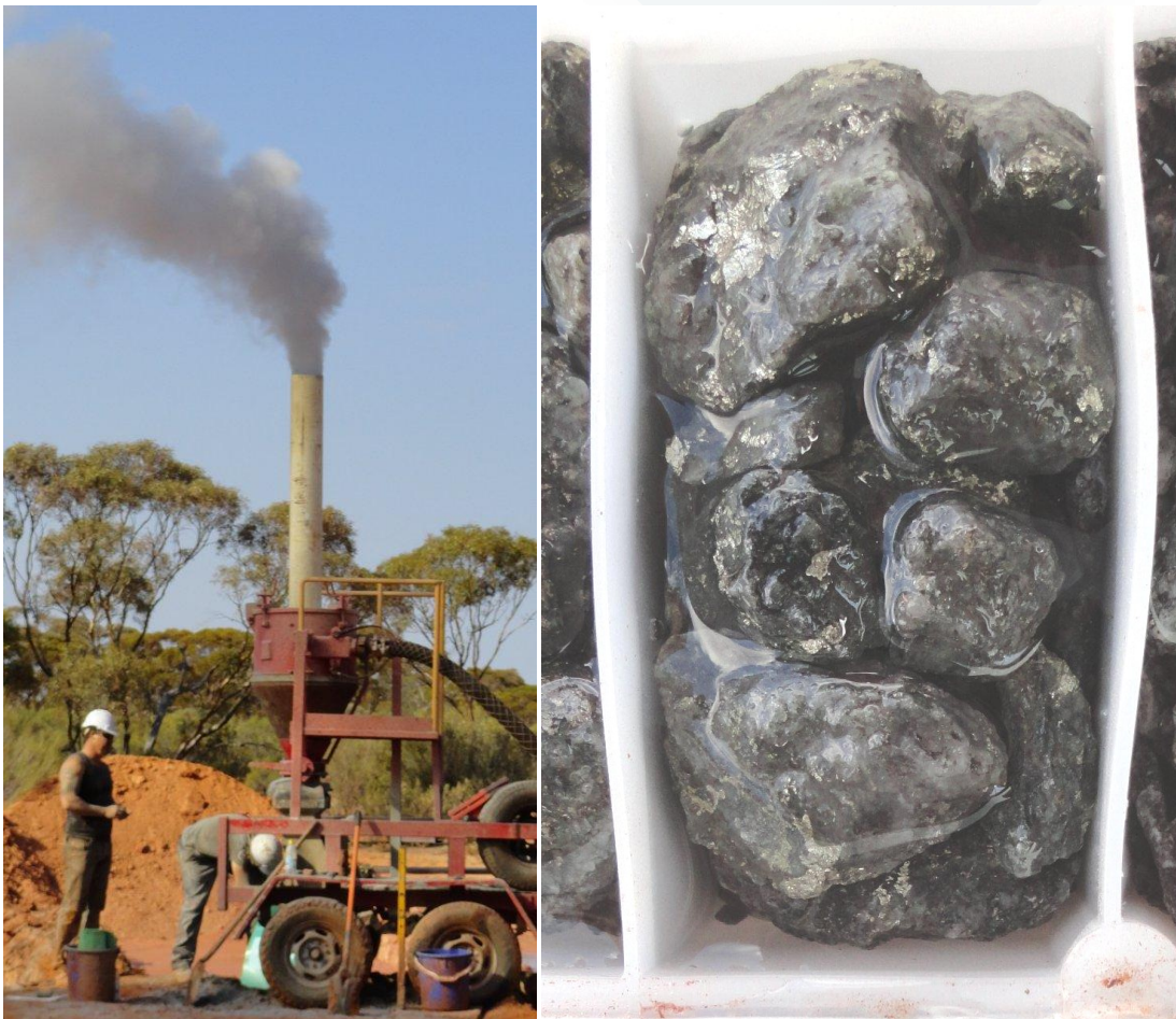
Photos: left – sample cyclone and splitter Sept. 2012, grey dust is indicative of sulphides in bedrock. right – altered RC chips containing coarse disseminated pyrite in RCLR170.
