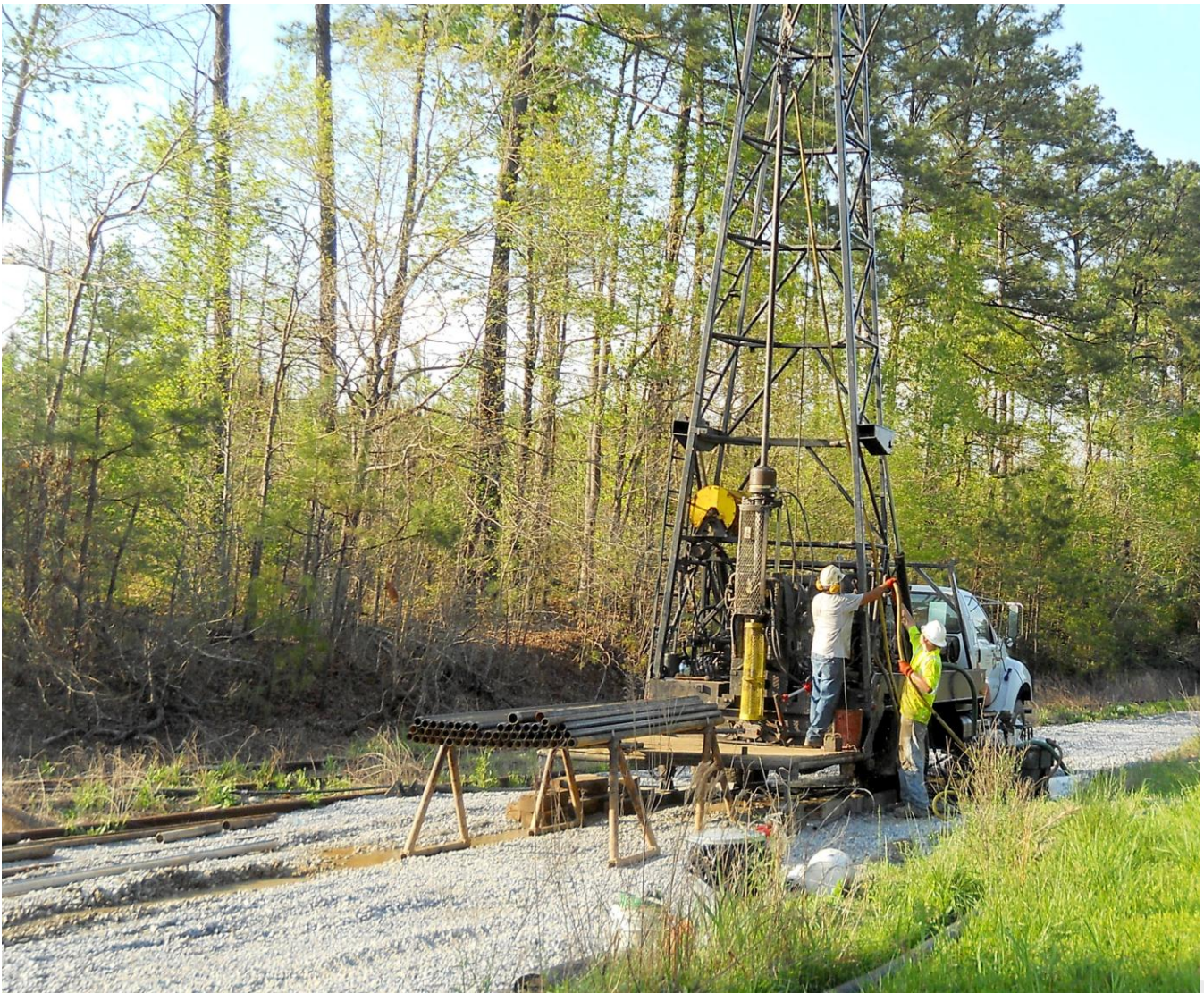
Fig 1: Boart Longyear diamond drill rig drilling at Kodiak Coking Coal Project, Alabama, USA.
