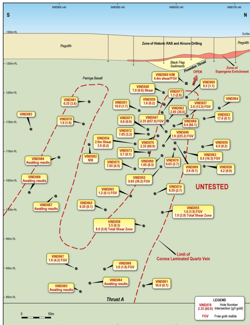
Figure 8: Corona long section showing exploration results received to July 2012. The hashed line shows the extent of the laminated quartz vein. A second shoot of laminated quartz has been identified to the south of the main shoot where the majority of assay results are still awaited. Downhole widths are shown with true widths estimated at 60-70% of downhole width.
