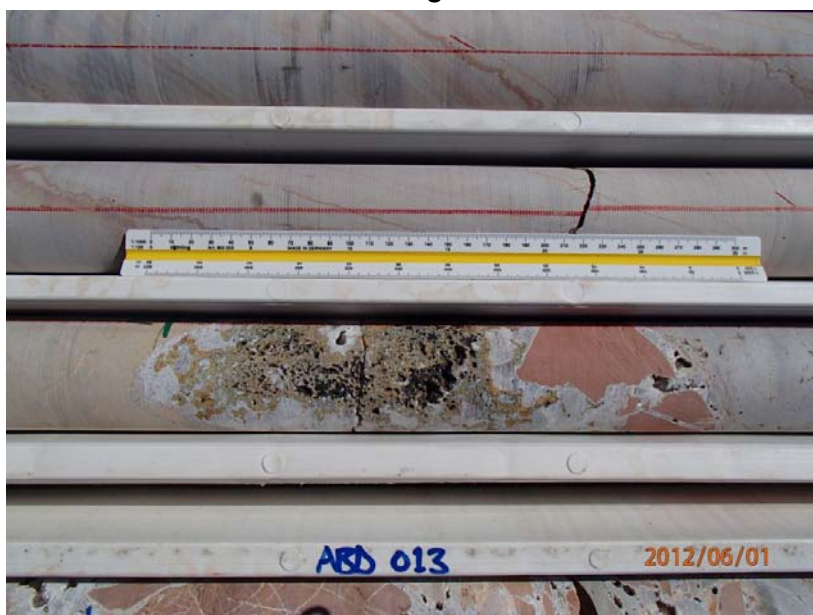
Figure 4: Descloisite-quartz vein intersected in ABD013 at 164.2-164.5m.
