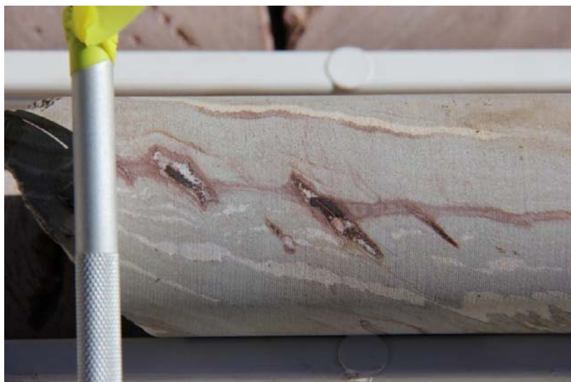
Figure 3: Parasitic folding within limestone footwall of descloisite mineralisation with sulphide mineralisation in ABD014 at 203m.
