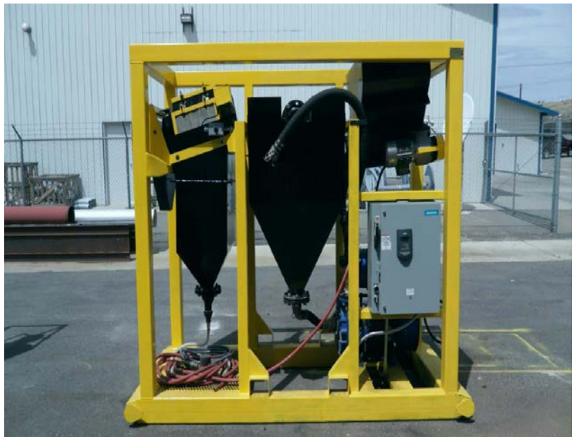
Pilot-scale Ablation unit capable of processing ~0.5 tonnes of ore per hour
