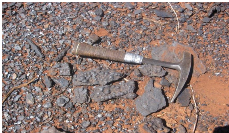
Figure 4 Botryoidal manganese slabs of up to 5cm in thickness occur within the Ilgarari Shale. Photo taken just outside the western boundary of Bligh's tenement
