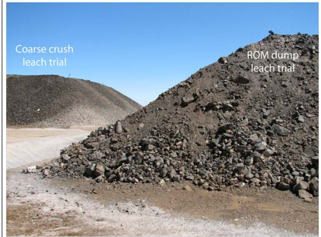
Figure 13.2.1_1 First ROM and Coarse Crush Leaching Trial
