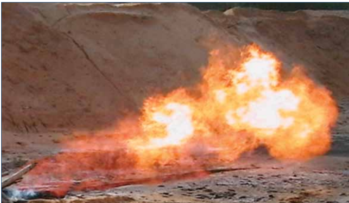
Gas flowing during production testing at Advent's Waggon Creek-1 well in EP 386.
