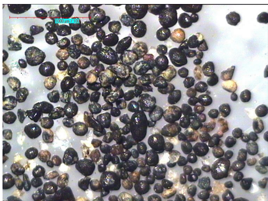
Figure 14: Microscopic pictures of concentrate (binocular 100 x magnification)
