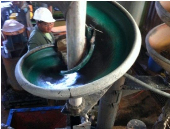
Figure 10: Spiral in operation. Beneficiated product is the dark colour (inside) and the shell fraction is the light colour (outside)
