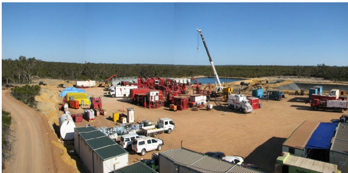
Fig 3. Arrowsmith-2 location with frac spread and all ancillary equipment in position
