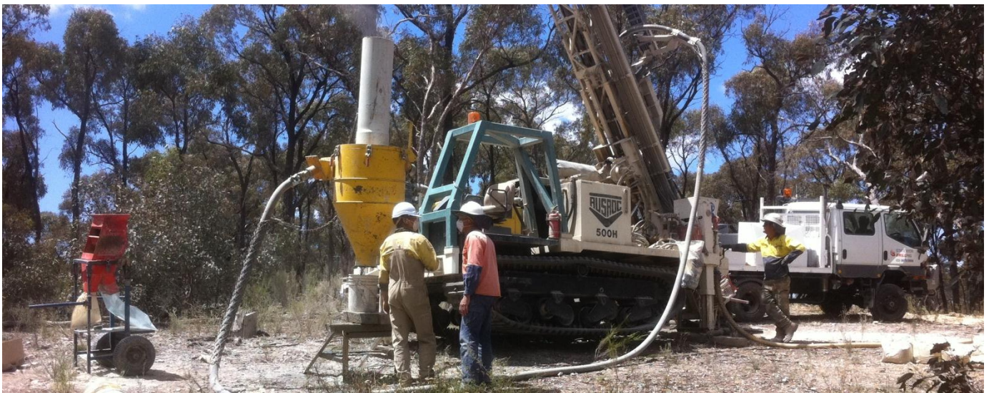
Reverse circulation drilling at Specimen Reef
