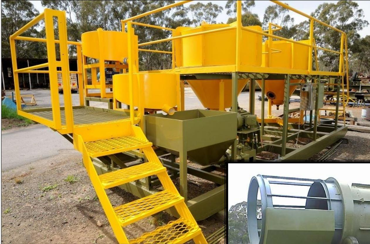
Twin 50 tph In-line Jigs with Spinners for heavy mineral and gold separation
