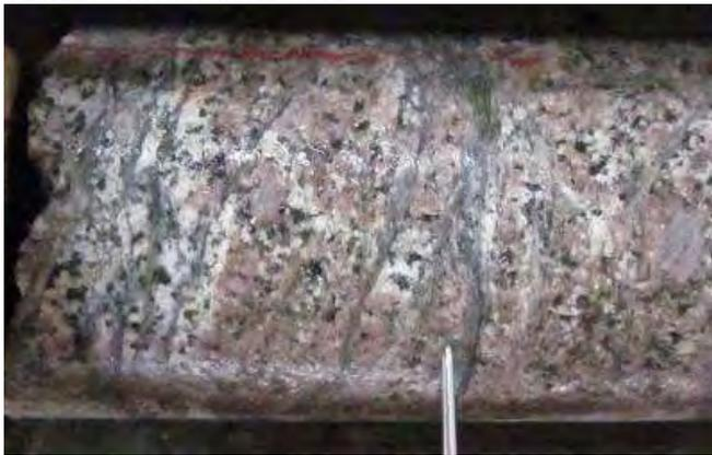
PLATE 10. WDD-016 230M: CLOSE-UP OF SILICA VEINS WITH CHALCOPYRITE – BORNITE – MAGNETITE INFILL IN DRILL CORE
