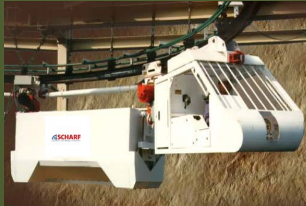
Monorail Train, high gradient, 10-30 tonne payload
