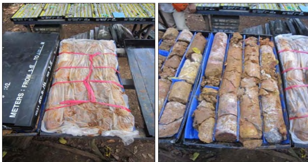
Figure 23: Core Trays With and Without Packing Bags and String to Ensure No Core Loss
