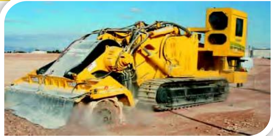
Simple quarrying using Vermeer equipment
