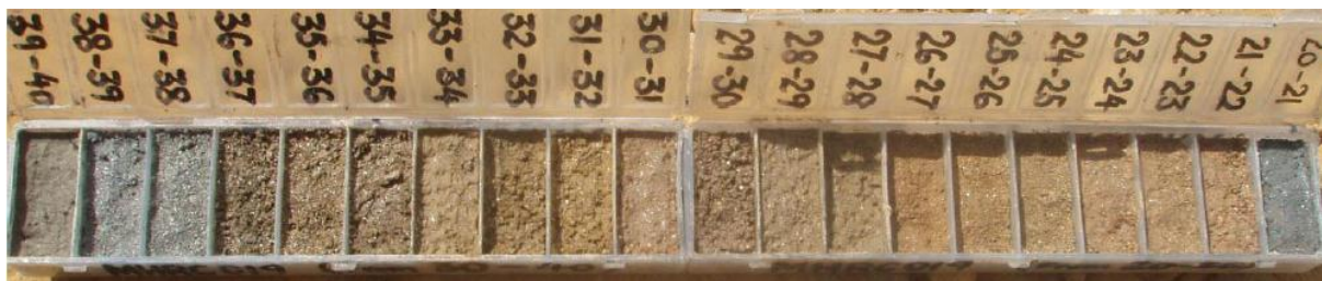
Figure 2: Graphite Mineralisation within hole MHRC019 at Epanko. (Assays pending).
