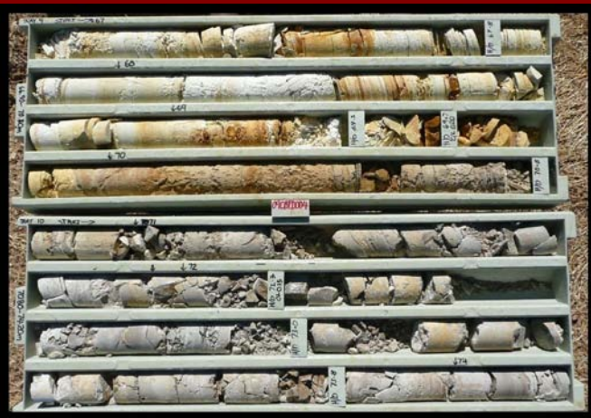
Diamond hole 09CBPD004 showing the high grade (36% P 2 O 5 ) ore zone from about 70m to 74.2m
