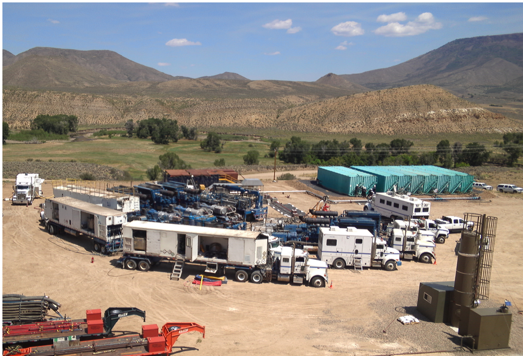
Photo showing fracture stimulation operations at Battle Mountain 14-10
