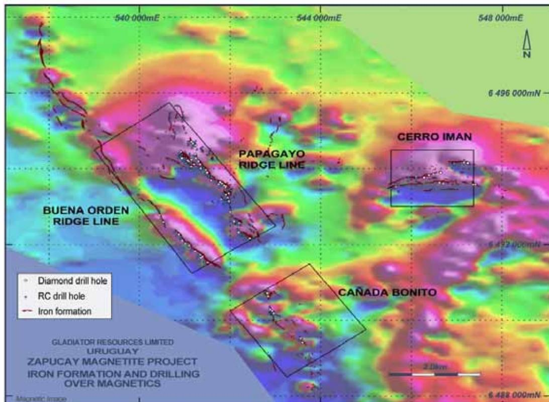
Figure 3: Project area showing drilling on a background of airborne magnetic survey
