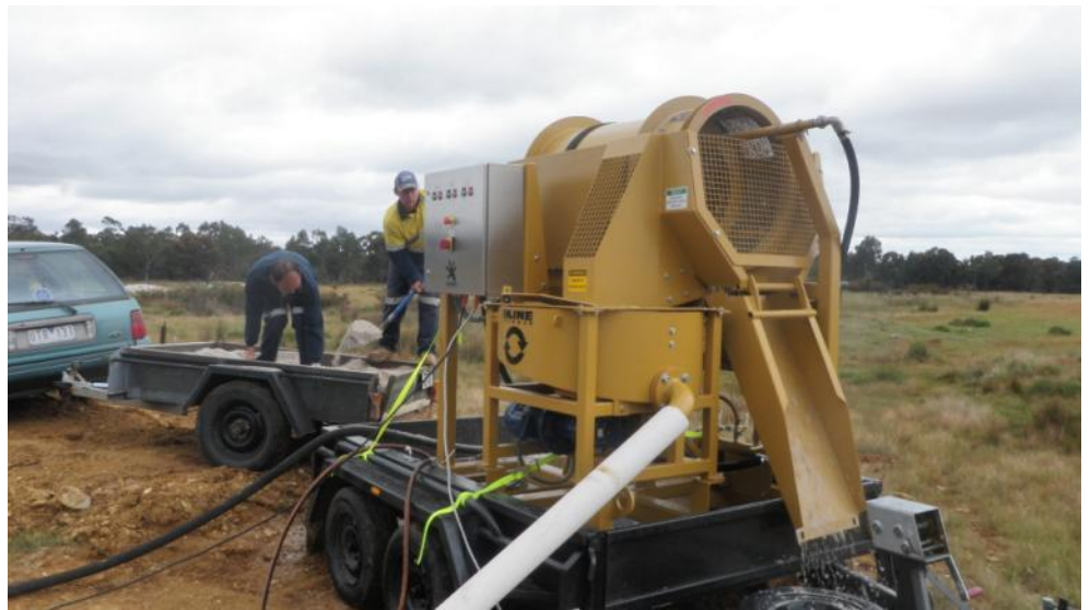
Gekko Test plant used to test for coarse gold from RC chips at Gowks Hill
