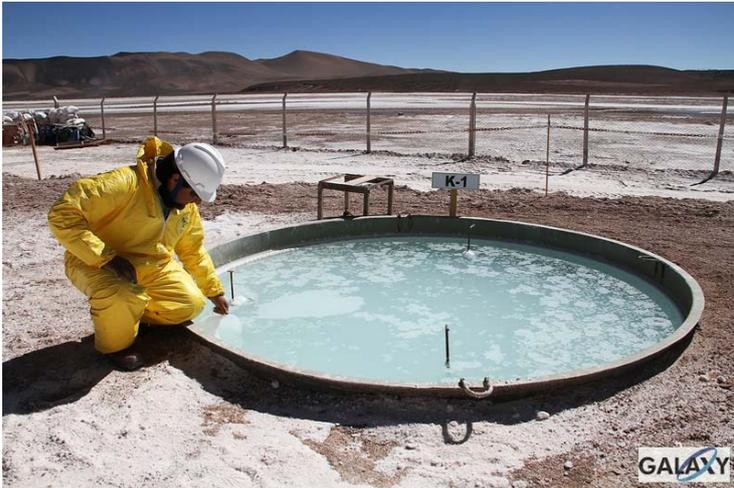
Evaporation test ponds being monitored
