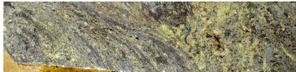
Copper mineralisation (yellow) at 235m downhole depth in diamond drill hole 09ATD015
