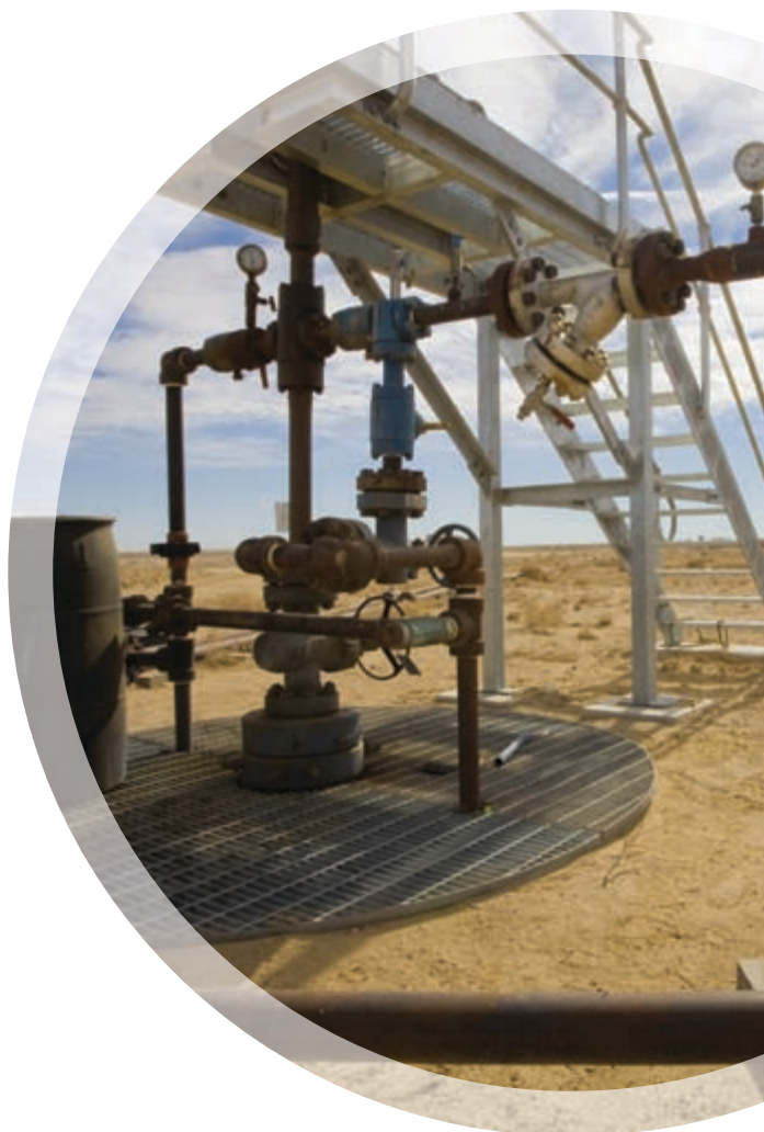
Above: Wellhead facilities for oil production - Cooper Basin SA
