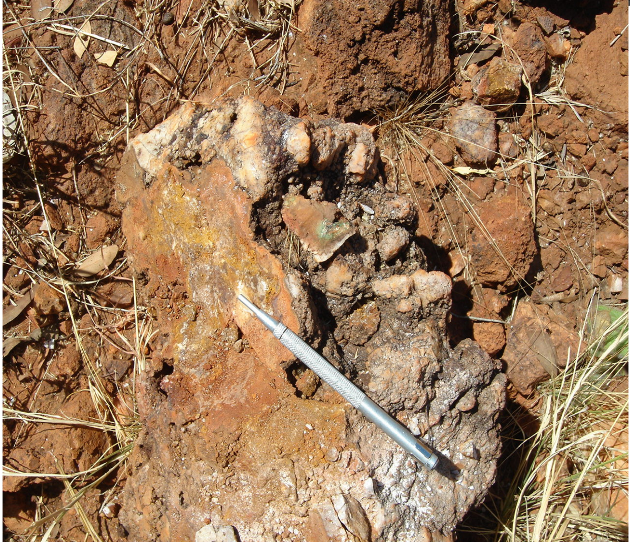
Fig. 4 Malachite staining associated with iron oxide-quartz breccia in the northwest of Area 3.
